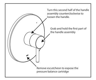
2. Remove escutcheon, threaded nipple and stem extension from the valve. See parts diagram.
